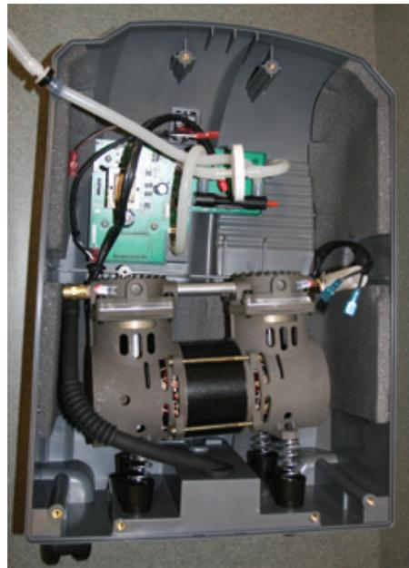
7. Lift the compressor upward from the bottom of the case to remove it from the concentrator.
