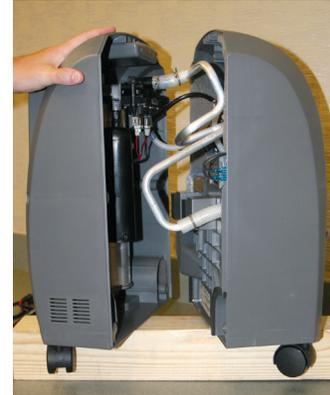
4. Disconnect the HEPA filter from the outlet barb tubing.
