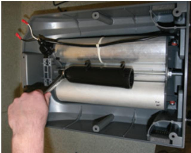
4. Pull outward on the top of the sieve bed assembly to remove it from the grommet at the top of the case.
