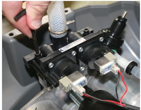
5. Pull outward to remove the 4-way solenoid assembly.
