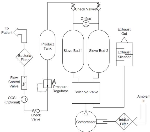
Figure 3: Schematic Diagram of Pneumatic Operation
