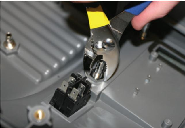
5. Pull outward on the flow meter from the outside of the concentrator to remove it.
