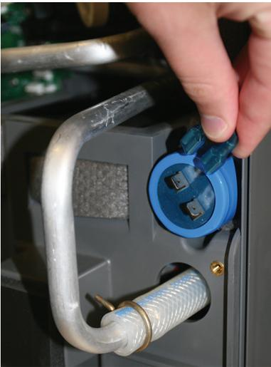
4. Pull upward to remove capacitor.
