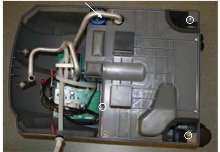
5. Pull outward to slide the compressor cover out from the body of the concentrator.
