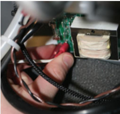
7. Cut zip tie securing all wires together.
