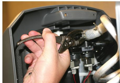
4. Disconnect the braided tubing from the 4-way solenoid.
